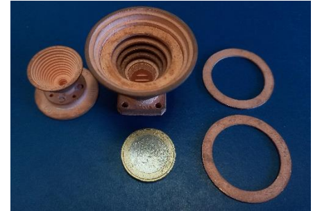
Fig. 1: Conical Horns build base and corrugated using FFF
