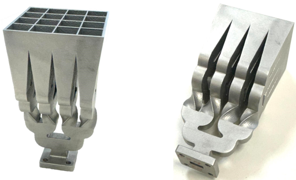
Fig. 2: Photographs of the additively manufactured difference pattern horn array antenna in AlSi10Mg.
