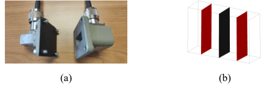
Fig. 2. (a) Waveguide measurement setup. (b) CST MWO simulation.
